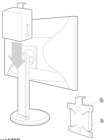
Use the felts as shown in the figure above and slide the MD BRPCV02 bracket with the mounted device on top of the stand of a compatible iiyama height
